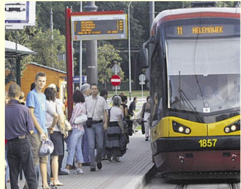
New PESA 122 (10) and electronic system of displays presenting arrival and departure schedule
